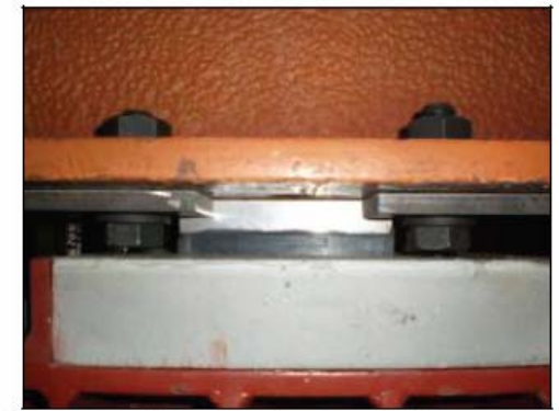
Figure 6 Installation of bearing
